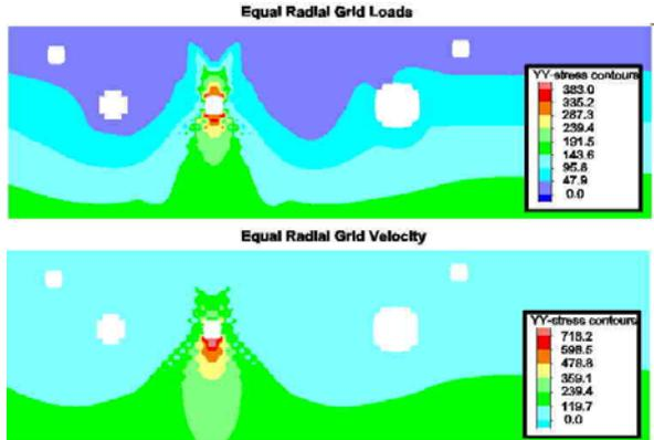
Figure 4. Vertical Stresses (kPa) due to pipe bursting.
