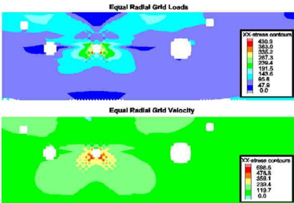
Figure 3. Horizontal Stresses (kPa) due to pipe bursting.
