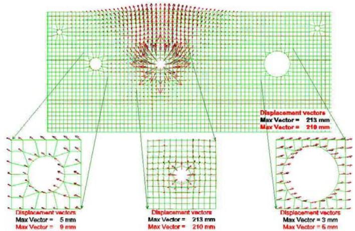
Figure 2. Deformation pattern in the vicinity of the burst pipe. The black (upper) and the red (lower) values indicate the results of the first and second models, respectively.
