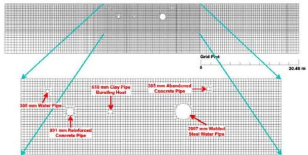
Figure 1. Existing utilities relative to the pipeline to be burst.
