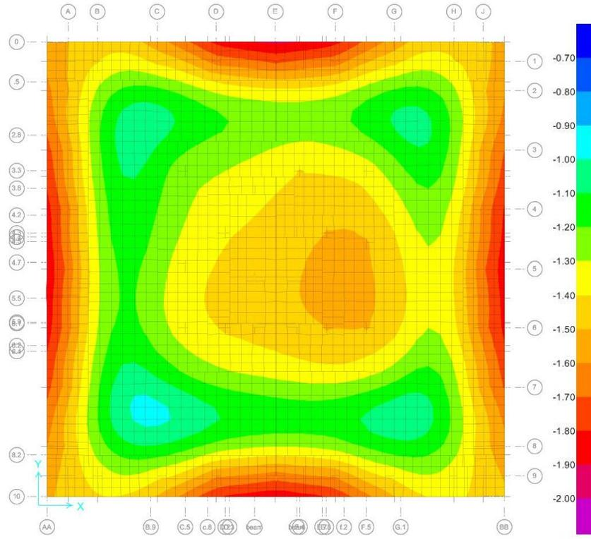
Figure 2- Mat slab settlement contours in centimeters under 100% of dead loads for  $k_s = 15.5 \text{ MN/m}^3$  (57 lbs/in<sup>3</sup>)
