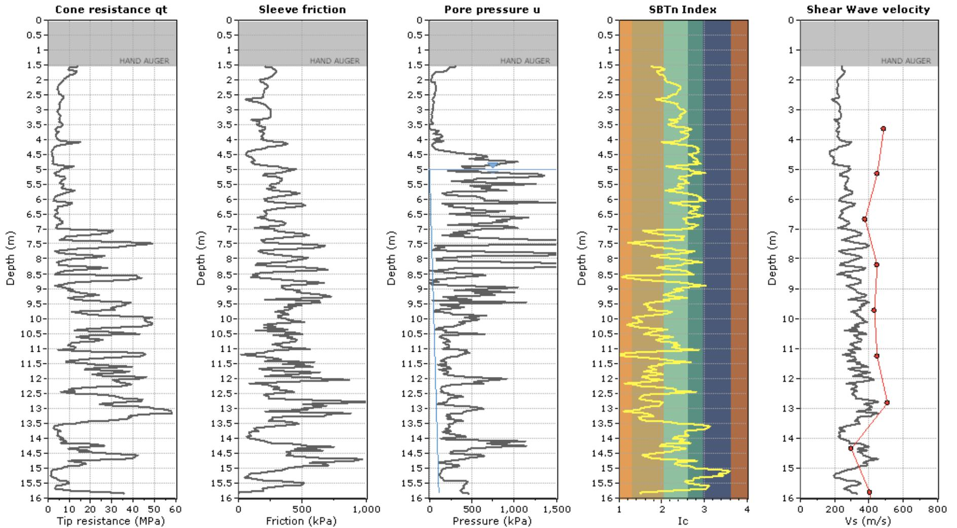
Figure 1- Representative CPT profile of the Terrace Deposits over the soft rock with the measured shear wave velocities.
