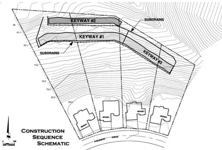
**FIG. 7. ACS Keyway Locations and Construction Schematic**
