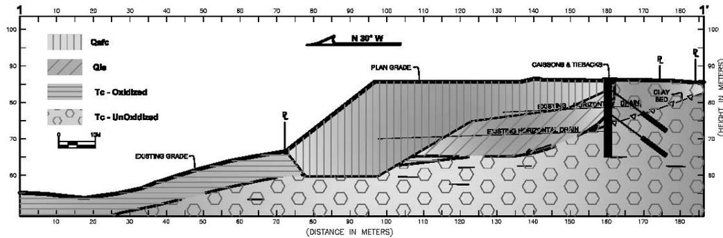
**FIG. 5. Cross Section of Keyway/Toe-Surcharge Repair Option**
