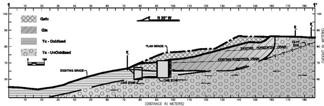
**FIG. 6. Cross Section of ACS Repair**
